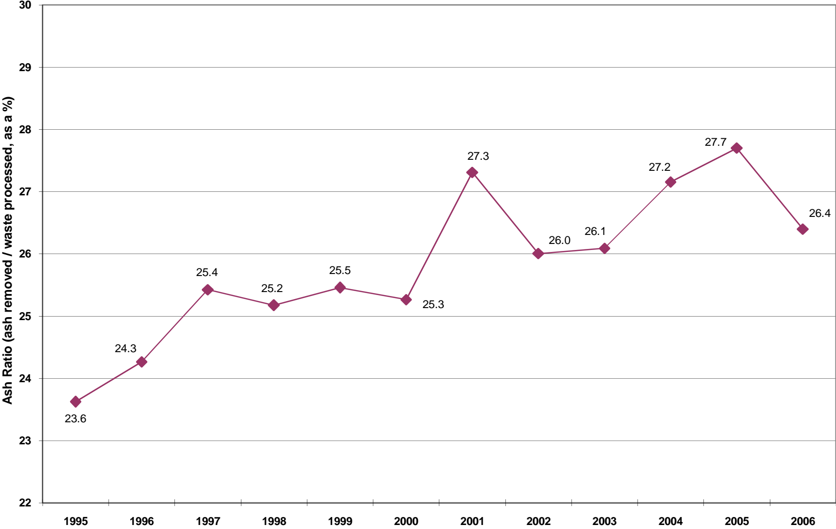
Figure 5. Annual Average Ash Ratio as Percent of Throughput Onondaga County Resource Recovery Facility
